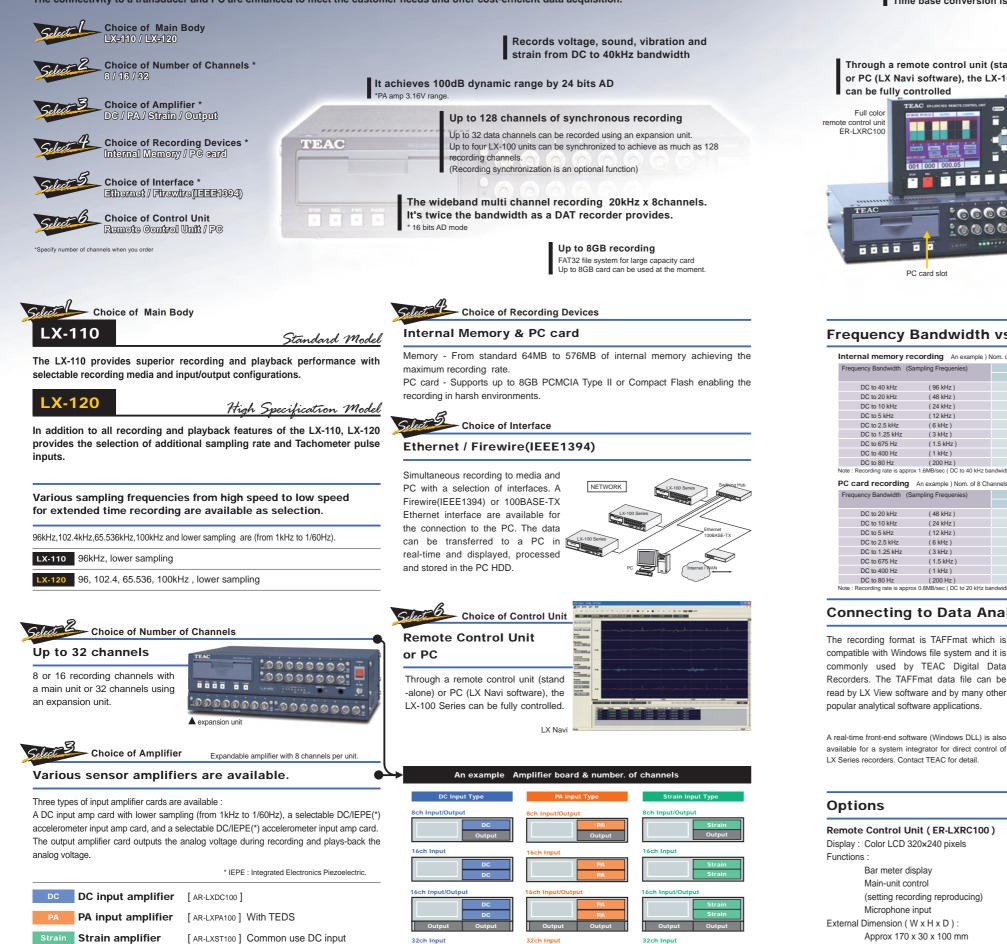
Time base conversion is possible in playback. Recording format is TAFFmat, which is supported by many popular analysis software applications. Through a remote control unit (stand-alone) or PC (LX Navi software), the LX-100 Series can be fully controlled
